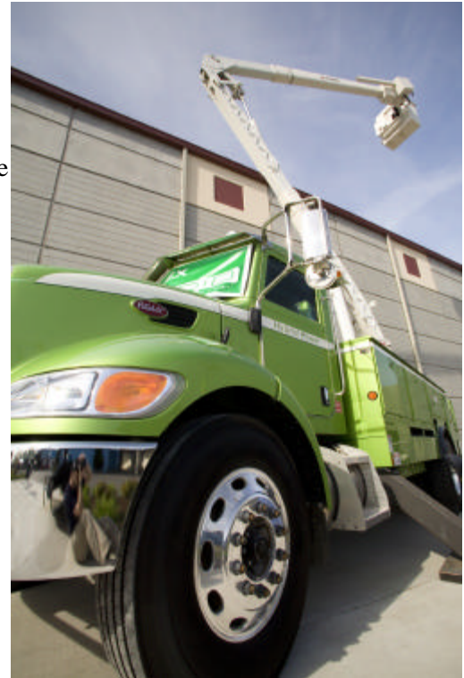
Crowds jammed the Clark County fairgrounds during the weekend Clark Public Utilities' Home and Garden Idea Fair. Also at the fair were large numbers of hybrid vehicles, including Hondas, Toyotas and Mercurys and the Peterbilt hybrid-diesel bucket truck, above. Diesel engine truck generates electric power to operate extendable bucket saving fuel during operations.
