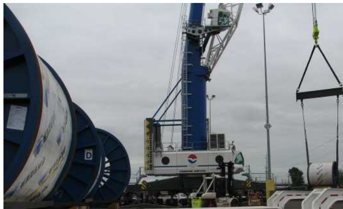
Port of Vancouver's behemoth mobile crane, largest in North America, offloads 90-metric-ton reels of cable for trip to Vancouver, B. C. to become part of the largest ski lift in world for the 2010 Winter Olympics.
